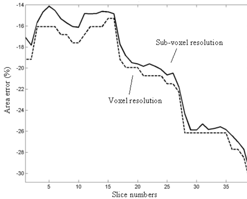
Figure 5.10: Area errors of the method running in voxel resolution and the approach using the level set methods running in sub-voxel resolution. This figure shows that the errors of area estimation are -21.24\% and -20.27\% for the methods running in voxel and sub-voxel resolution respectively, and reveals that the accuracies of the sub-voxel based method and the voxel resolution method are comparable.
