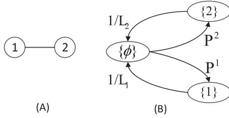
Fig. 6. A network with two nodes and its corresponding continuous Markov chain.
