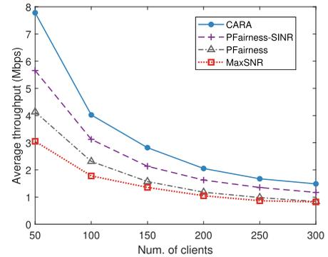
Fig. 14. Throughput versus client number.
