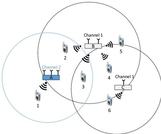
Fig. 1. A wireless network formed by APs with heterogeneous numbers of antennas. The channel assigned to each AP is labelled at the top of the AP.
