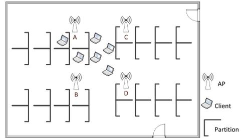
Fig. 20. Locations of APs and clients for the 802.11n testbed.
