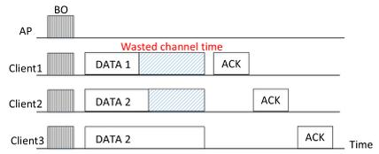
Fig. 5. Downlink transmission scheme with fixed size packets
