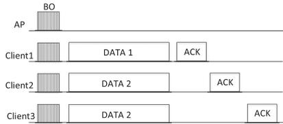
Fig. 4. Downlink transmission scheme with fixed duration
