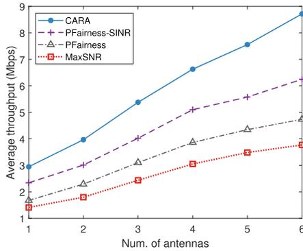
Fig. 11. Throughput versus antenna number.
