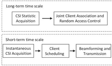
Fig. 2. Block diagram of long-term and short-term operation of the system under study.
