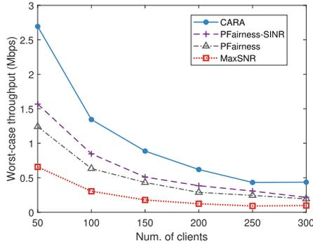
Fig. 16. Worst throughput versus client number.
