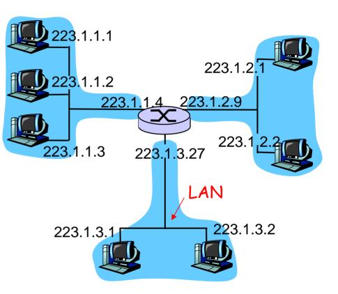
network consisting of 3 subnets (for IP addresses starting with 223, first 24 bits are network address)
