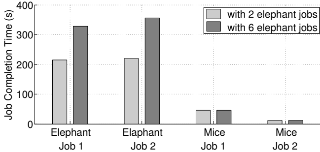
Fig. 7: Comparison of completion time of two elephant and two mice jobs, running with and without four additional elephant jobs, respectively.
