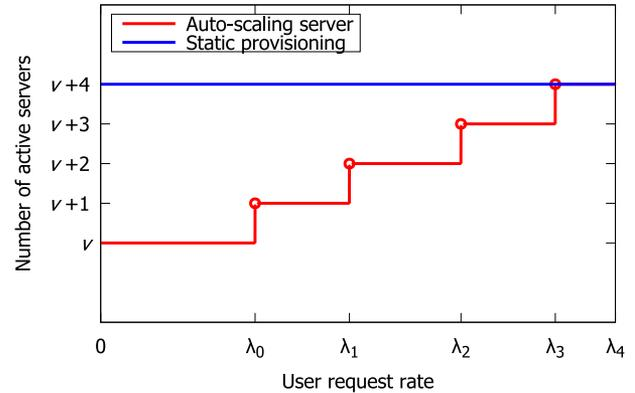
Fig. 2. Mapping mechanism of auto-scaling levels.
