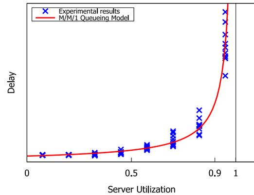
Fig. 3. Delay model for an auto-scaling server.
