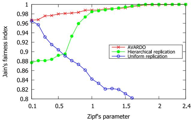
Fig. 9. Utilization fairness versus Zipf's parameter of block access probability distribution.
