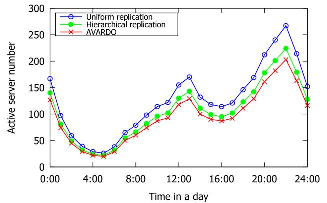
Fig. 11. Number of active servers over a typical day.
