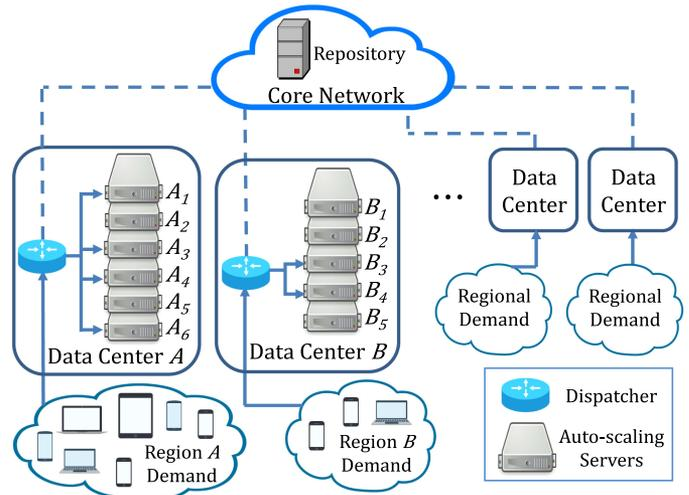
Fig. 1. A video cloud consisting of auto-scaling VoD data centers.
