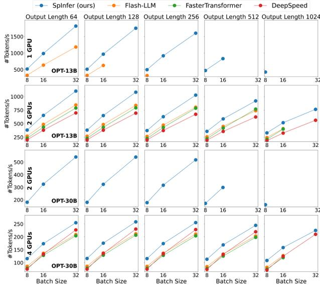
**Figure 13.** End-to-end inference performance of OPT-13B and OPT-30B on RTX4090 GPUs.
