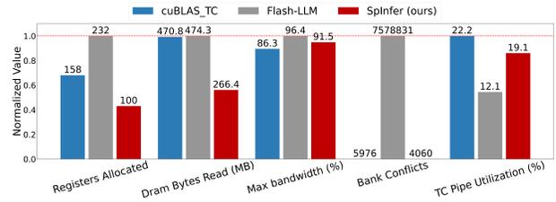
Figure 12. Micro-level comparison of SpInfer against cuBLAS\_TC and Flash-LLM across key metrics.
