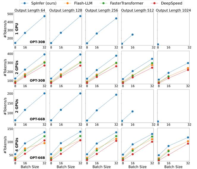
**Figure 14.** End-to-end inference performance of OPT-30B and OPT-66B on A6000 GPUs.
