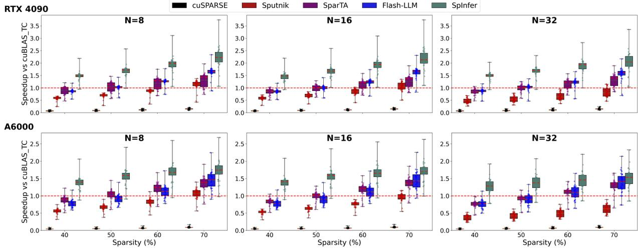
Figure 10. SpMM kernel performance comparison on RTX4090 and A6000 GPUs.  $N$  denotes the batch size.
