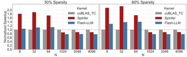
**Figure 16.** Performance comparison under small and large N settings.  $M = 28672$  and  $K = 8192$ .
