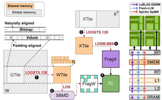
Figure 7. Data movement and instruction pipeline.
