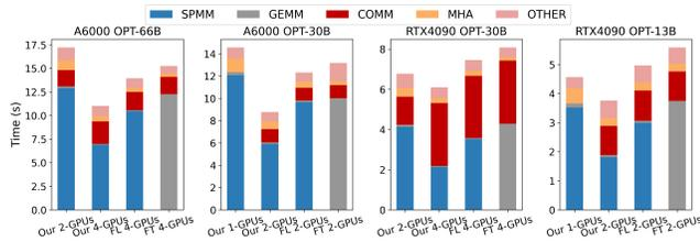
**Figure 15.** Breakdown of end-to-end inference time. FL: Flash-LLM. MHA: Multi-Head Attention. COMM: Inter-GPU Communication.
